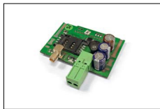
Modem GSM e internet GPRS (COMAP) GSM modem and internet GPRS (COMAP) Modem GSM et internet GPRS (COMAP) Modem GSM e internet GPRS (COMAP)
